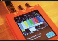
SyncVV supports a variety of input video formats, greatly reducing the burden of selecting video equipment in the field. Supported video formats range from 60p to 23.98p for 2048x1080 progressive, 60p to 23.98p for 1920x1080 progressive, and 60i to 50i for 1920x1080 interlaced. 1280x720 from 60p to 23.98p, Supports a wide range of input video formats. Progressive segmented frames are also supported, making it suitable for use in sites where a variety of video equipment is connected.
